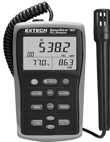
Fig.5: Indoor air quality meter
